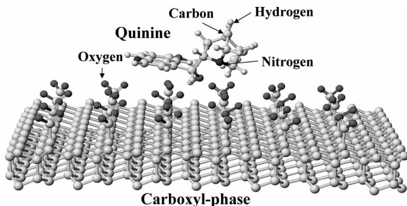
Figure 2. Docking of quinine on carboxyl-phase; small white ball: hydrogen; large white ball: carbon; large gray ball: oxygen; large black ball: nitrogen.
